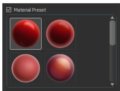
Surfaces are rendered with a “Material” that can be chosen from a list of “Material Preset”. Many of the “Material Preset” choices have bright edges highlighting regions where the surface normal is perpendicular to the line of sight. Some of the “Material Preset” choices add texture added to the surface. Please note the texture is a rendering effect and does not come from the original image data.
