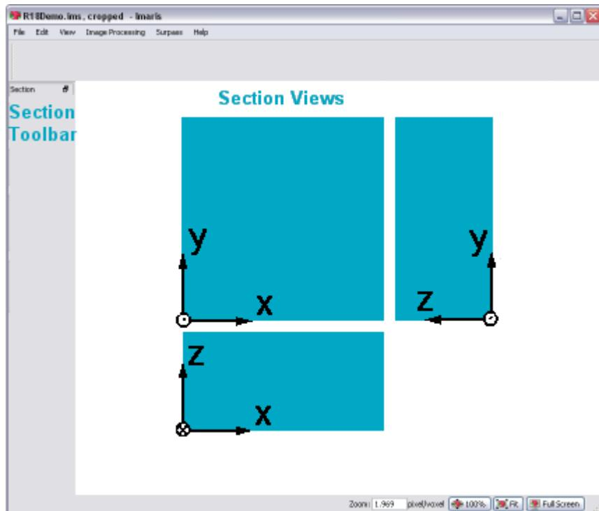
To select a point, click in any of the three views, hold the button down & drag the crosshairs to the requested point. The crosshairs immediately snap to the cursor when clicking anywhere in the image. The other views, connected by one coordinate, automatically follow the movements.
