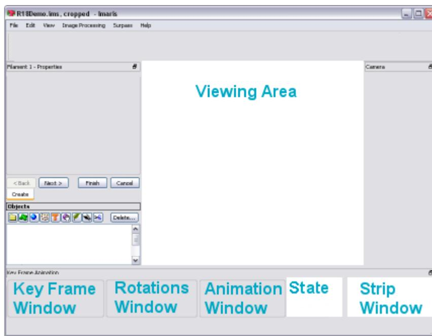
At the bottom of the screen the following windows are displayed: the [Key Frame Window](#), the [Rotations Window](#), the [Animation Window](#), the [State](#) selection, and the [Strip Window](#).
