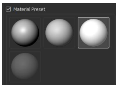
Spots are rendered with a “Material” that can be chosen from a list of “Material Preset”. Many of the “Material Preset” choices have bright edges highlighting regions where the surface normal is perpendicular to the line of sight.
