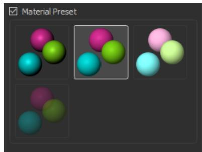
Cells are rendered with a “Material” that can be chosen from a list of “Material Preset”. Many of the “Material Preset” choices have bright edges highlighting regions where the surface normal is perpendicular to the line of sight.
