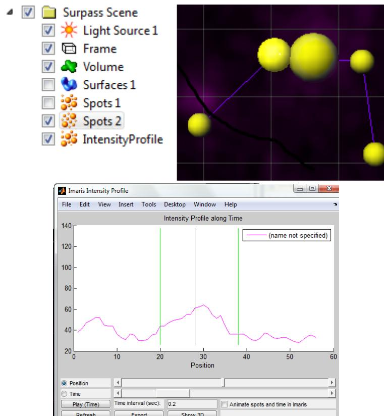
The channel colors are displayed in the plot. The intensities of the channels are shown using different colors respective to the channels. Several options allow the user to have control over the parameters of the calculation and how the results are displayed.
