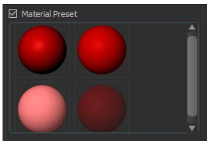
Filaments are rendered with a “Material” that can be chosen from a list of “Material Preset”. Many of the “Material Preset” choices have bright edges highlighting regions where the surface normal is perpendicular to the line of sight.
