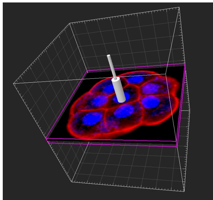
The position of the Oblique Slicer can be changed. Choose the pointer mode Select, highlight the Oblique Slicer in the viewing area and click on the bigger diameter rod. It will appear highlighted as it is selected, allowing you to move it and to set the Oblique Slicer to the required position.
