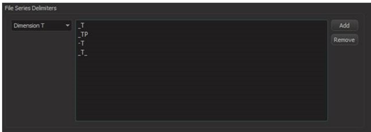
Dimension F (Split) is by default not detected automatically (it does not contain any default delimiter). Therefore to have File Series Split detected automatically, some delimiters must be added (e.g. \_F, \_F\_, \_FLD).
