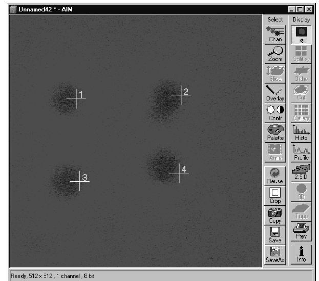
Fig. 5-398 LSM image of the Rh6G layer after bleaching. Deviations between the markers and the bleached spots are noticeable.
