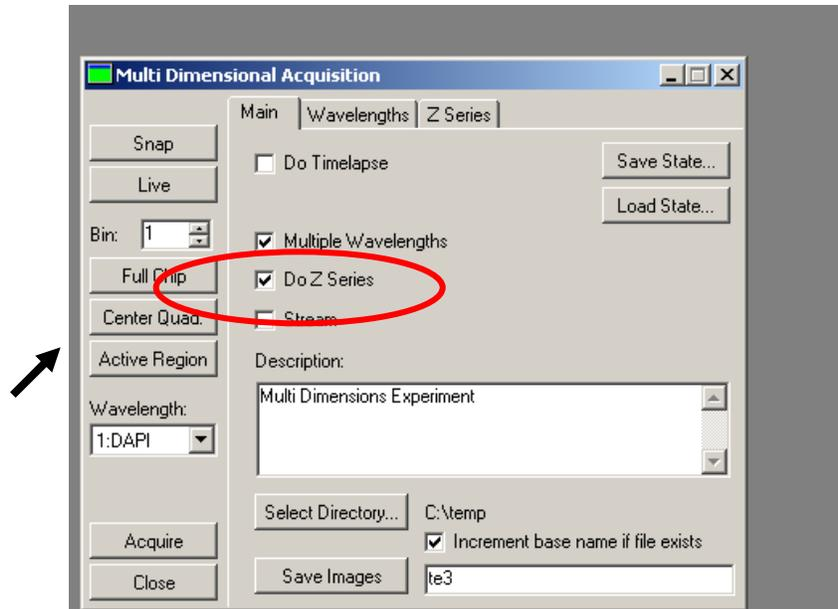
**Figure 6**, Multi dimensional acquisition window. For z-series, check **Do Z series** box
